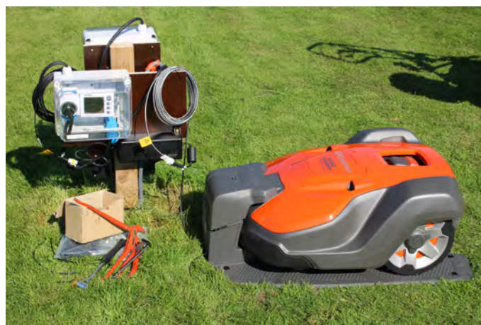
Photo 2: Husqvarna 550 automower in the ROBOGOLF project. At each charging station, a logger is installed to measure the energy consumption. Photo: Anne F. Borchert.
