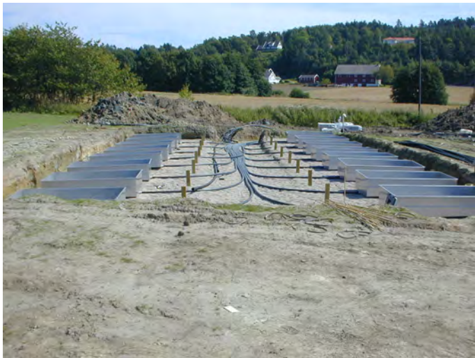
Photo 2: Most of STERF's studies on pesticide and nutrient leaching have been carried out in the USGA-spec. green field lysimeter facility at Bioforsk Landvik, Norway. Photo: Trygve S. Aamlid.
